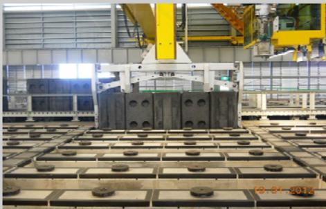
The overhead crane lifts 5 carbon anodes into the bake furnace.
