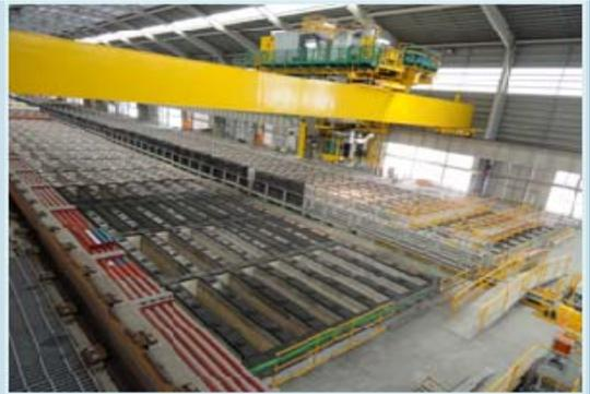
The 1.4 tonne 'green' (pre-baked) anodes are loaded into the furnace via crane and heated at temperatures over 1,200 degrees Celcius. The heating and baking process takes approximately 18 days, at which time they are removed from the bake and transported to the reduction cells for use as electricity conductors to make aluminium.
